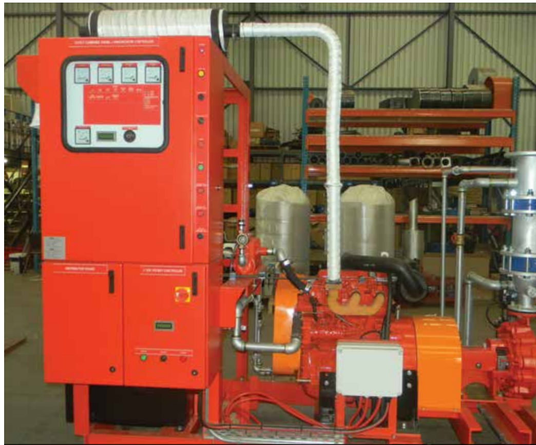
For customer Mega Pak in Zimbabwe, Gauteng fitted its KSB Etanorm 80-65-315 pump with a 31-kW (42-hp) John Deere PowerTech 2.9L GSPU engine.
